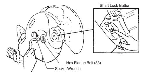
7. Remove the existing Saw Blade and replace with another 12 inch blade.
